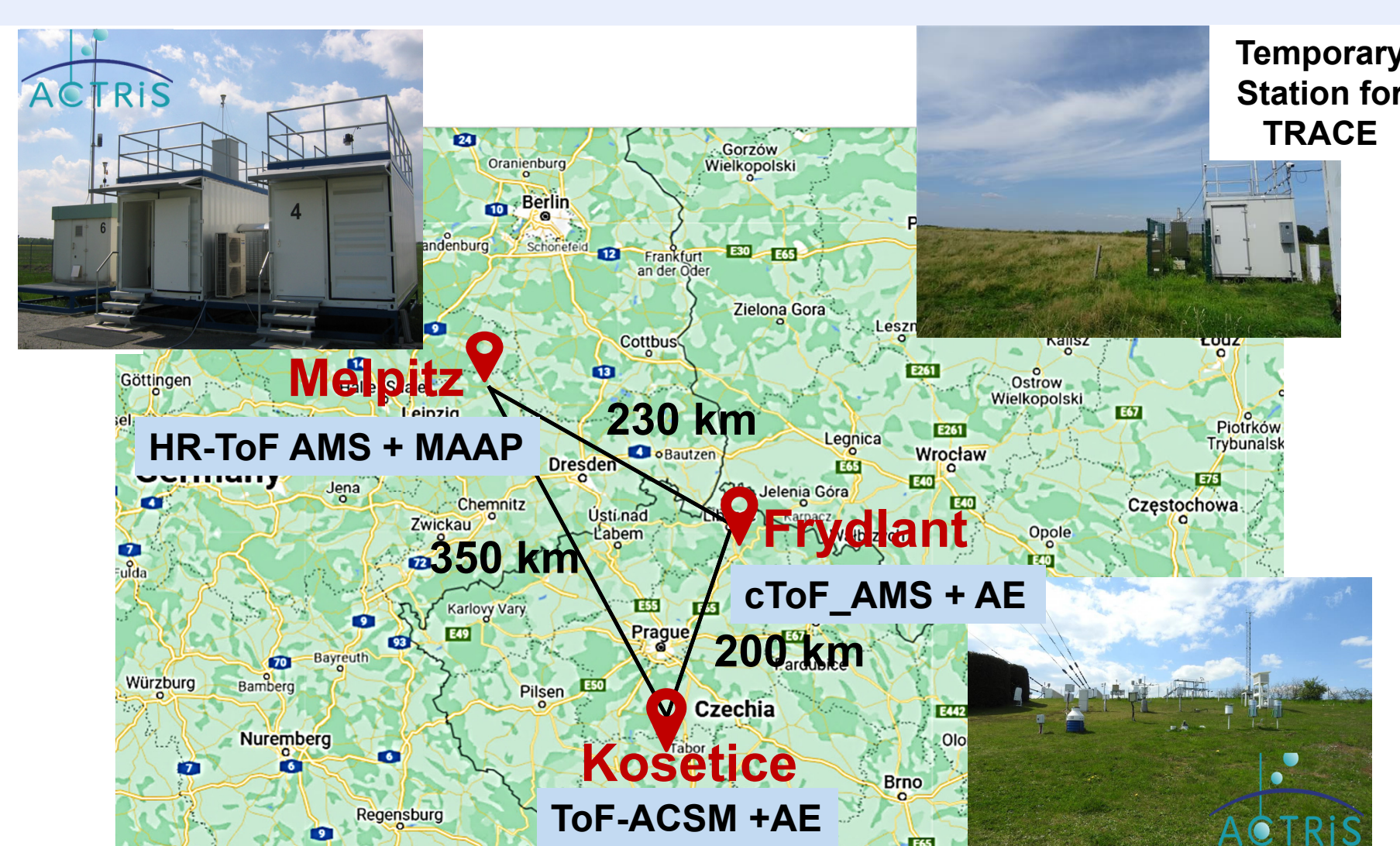
Fig. 1: The three TRACE measurement stations measure online aerosol chemical composition and black carbon and are equipped with high volume quartz digital samplers to measure PM 2.5
