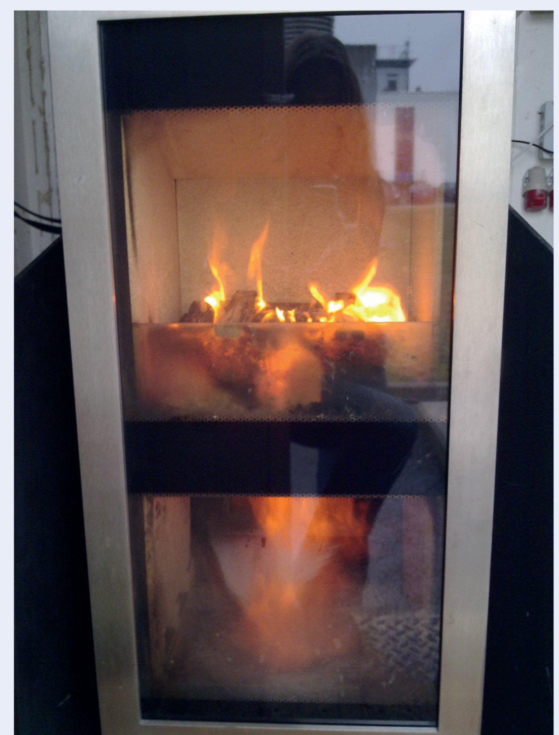
Fig. 2. Modern wood stove with two-stage combustion.
