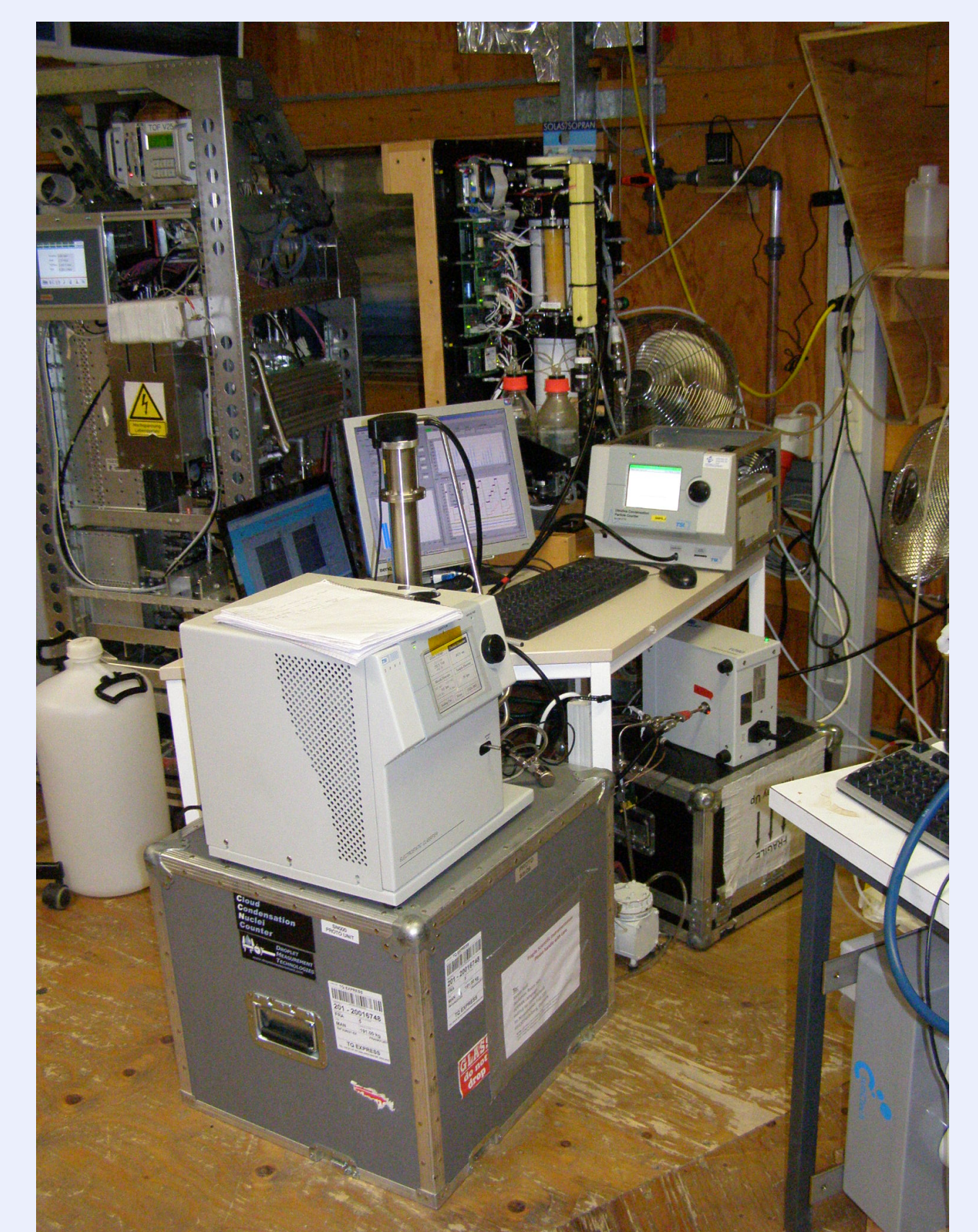
A schematic diagram and a picture of the experimental setup employed for online aerosol measurements.
