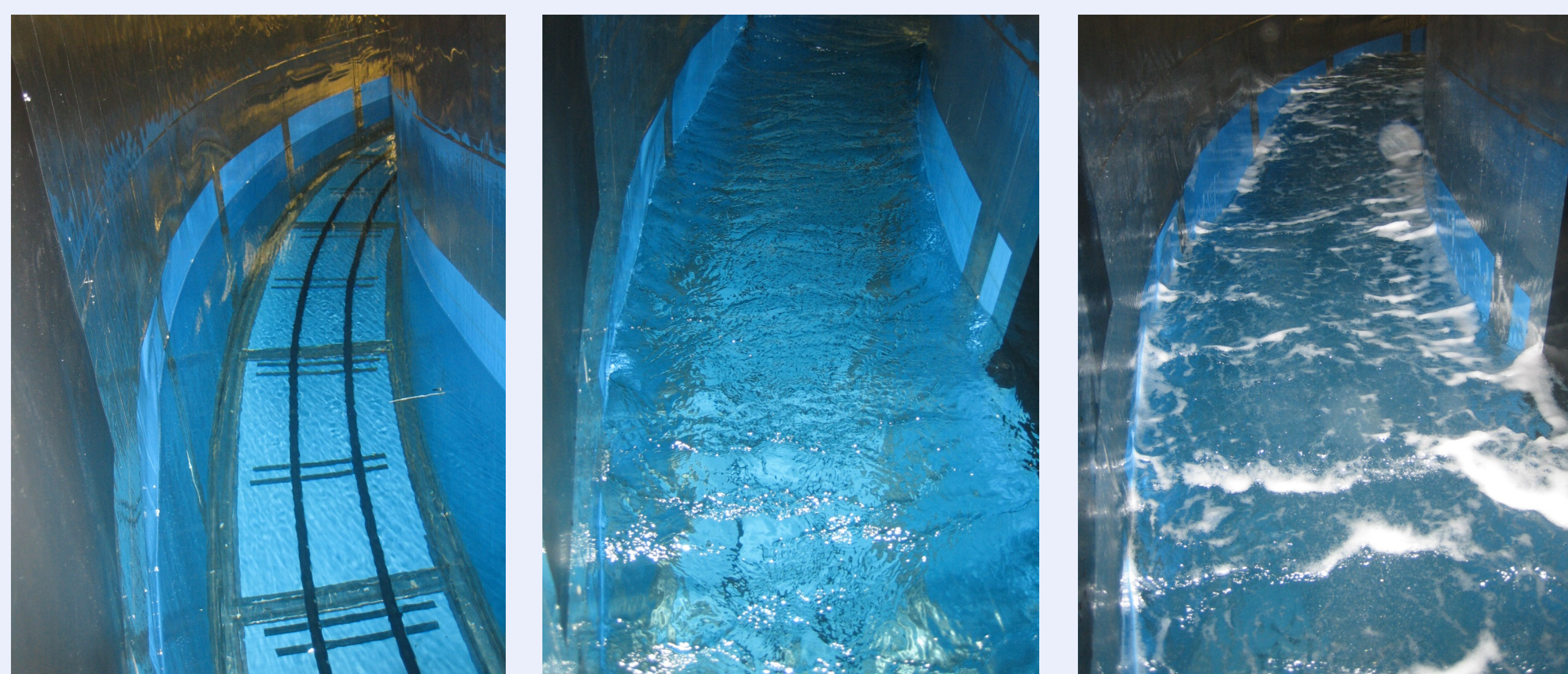
Wind speeds (u 10 ) of 5.21+/-0.34 m/s (left), 17.25+/-0.90 m/s (middle) and 13.7+/-1.3 m/s + bubbles from the aerator (right) in the Aeolotron.
