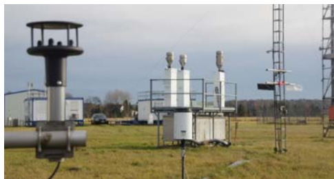
Figure 1: Measuring field of the TROPOS research site Melpitz (view to southeast). The HV-filter-samplers for daily samples on quartz fibre filter with inlets for PM 10 , PM 2.5 and PM 1 are shown in the middle of the picture.
