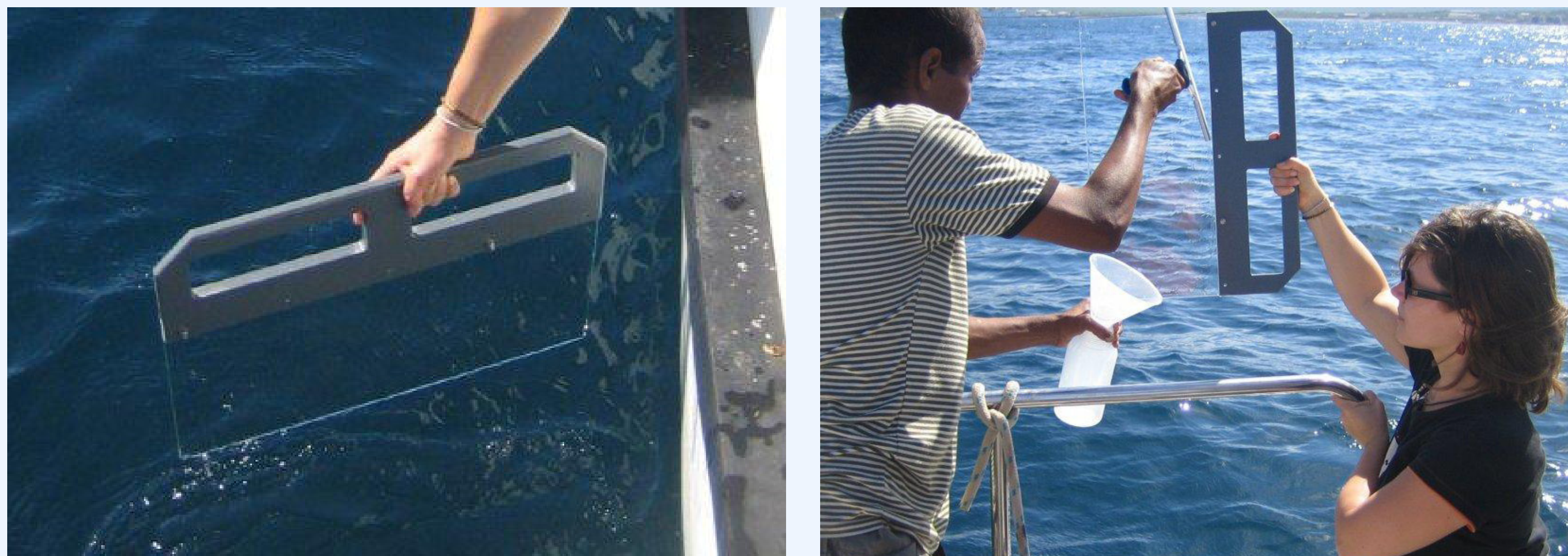
Fig. 2: Sampling of the SML using the glass plate technique, (left), Collection of the SML using Teflon Wipers (right).
