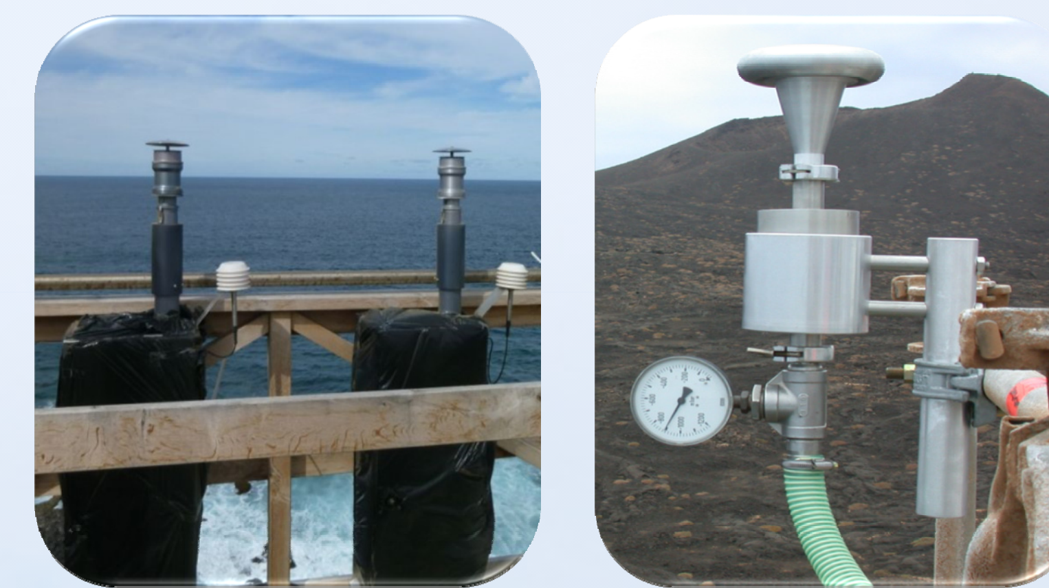
Fig. 3: a) Derenda low volume sampler with PM 10 -inlet, with 4 m 3 /h sampling rate on 47mm Teflon filters b) 5-stages BERNER impactor with 75 l min -1 , sampling rate on aluminum and Nuclepore® foil (Wicom Heppenheim GmbH, Germany), stages lower cut-offs: 0.05 - 0.14 - 0.42 - 1.2 - 3.5 - 10 µm.
