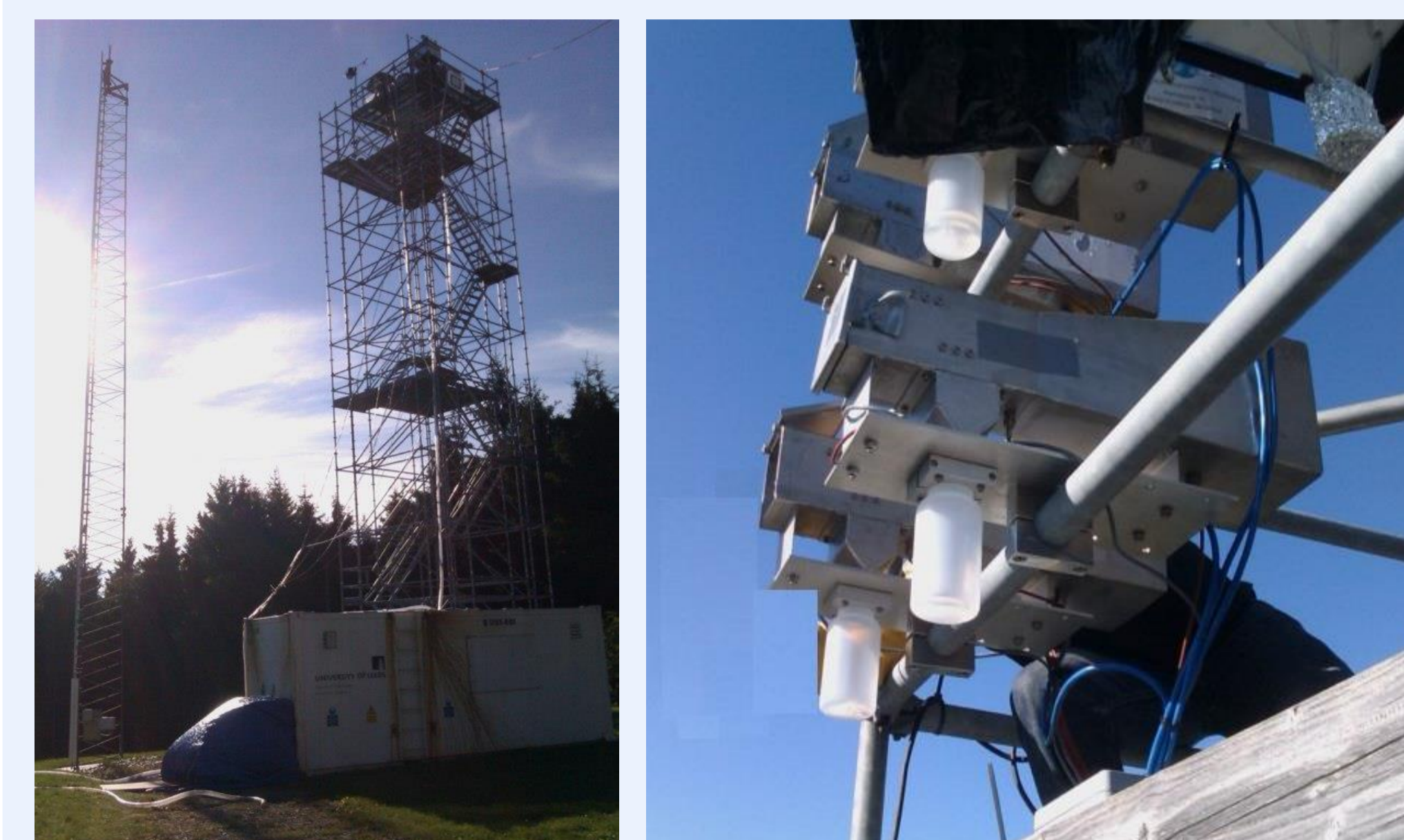
Fig. 1. Cloud water measurement tower during HCCT 2010 with collectors mounted at the sides at the top of the tower.
