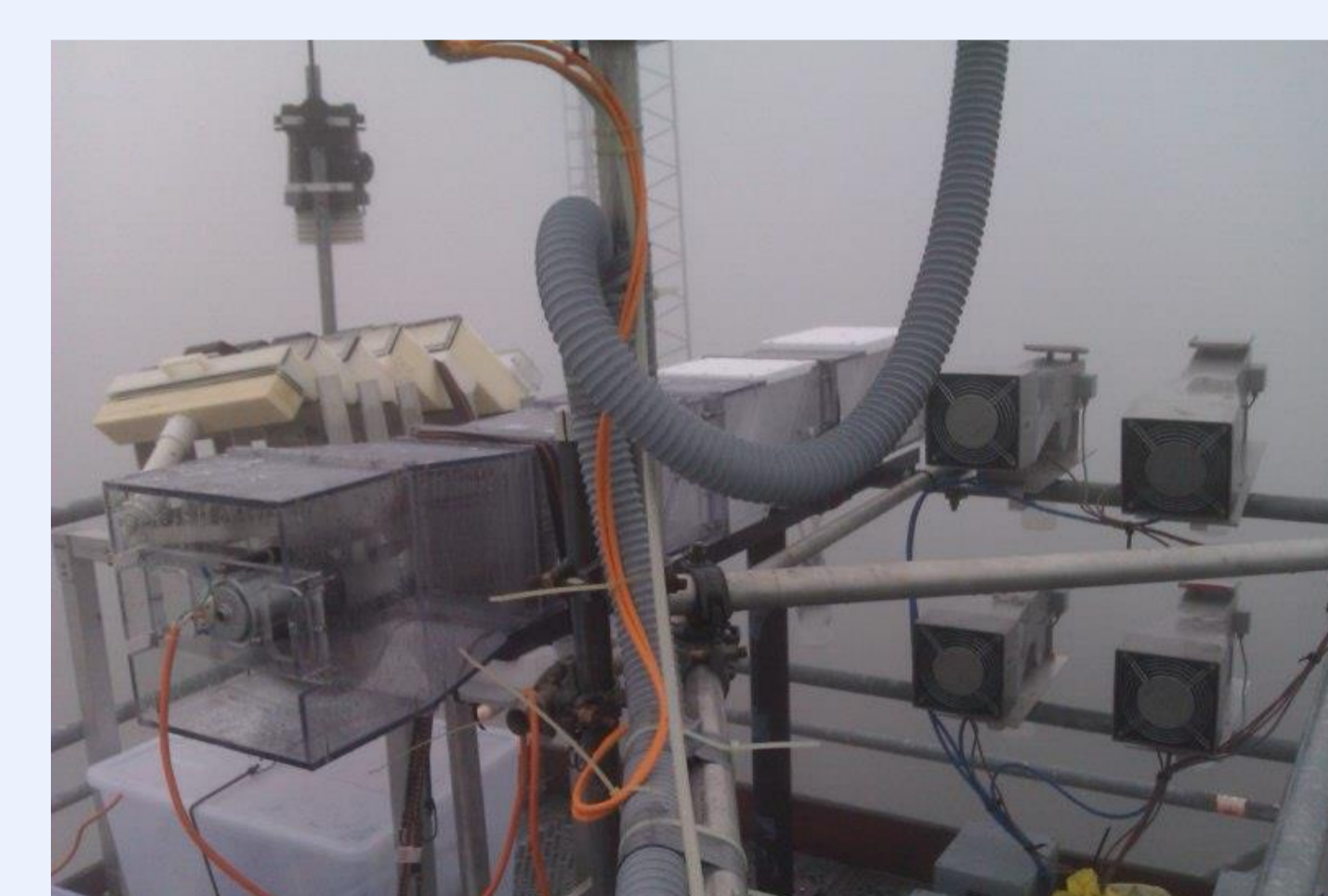
Fig. 2. Stainless steel Caltech Active Strand cloud water collectors on the tower platform during a cloud event
