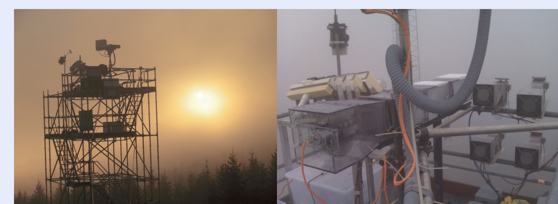
Figure 2: Pictures of the measurement tower and the cloud water collectors.
