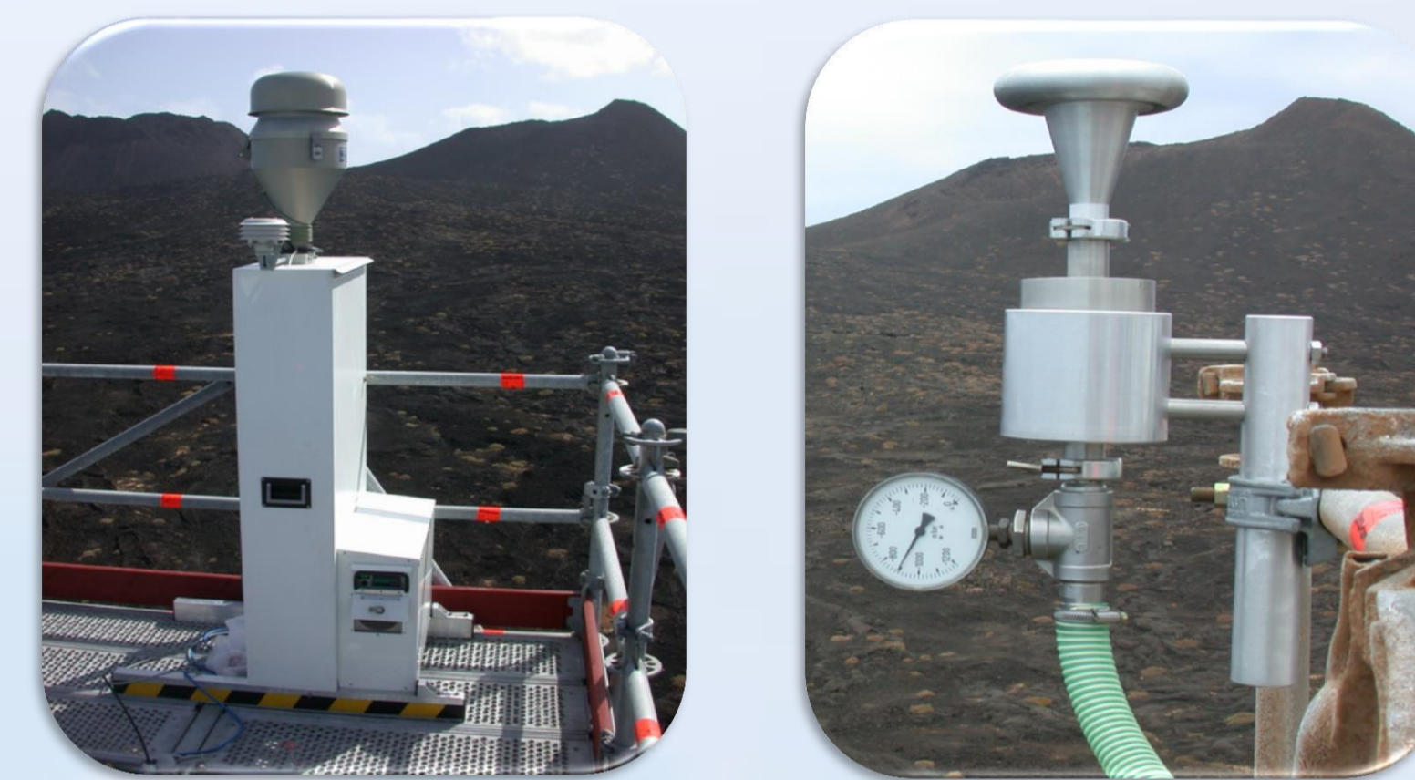
Fig. 3: a) Derenda low volume sampler with PM 10 -inlet, with 4 m 3 /h sampling rate on 47mm teflon filters b) 5-stages BERNER impactor with 75 l min -1 , sampling rate on aluminium and Nuclepore® foil (Wicom Heppenheim GmbH, Germany), stages lower cut-offs: 0.05 - 0.14 - 0.42 - 1.2 - 3.5 - 10 μm.
