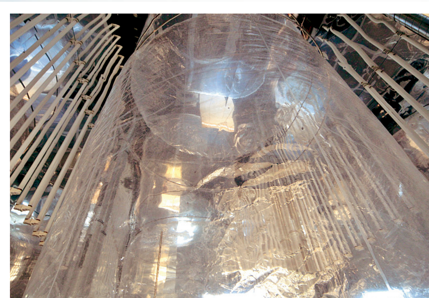
Fig. 2: The aerosol chamber surrounded by UV lamps
