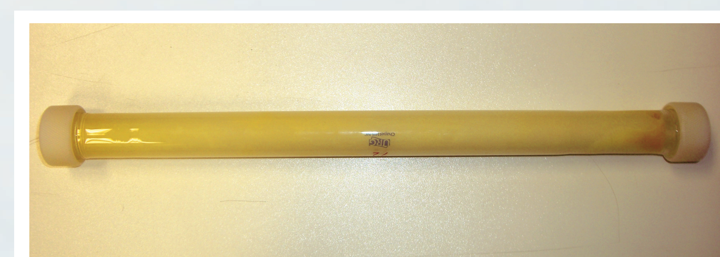
Fig. 3: Denuder coated with XAD-4 and DNPH
