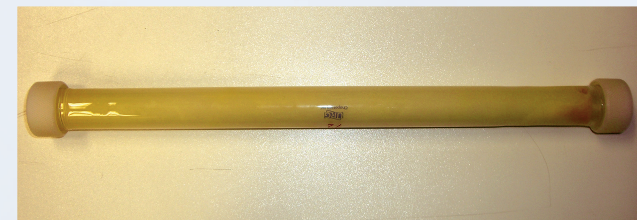
Fig. 2: Denuder coated with XAD-4 and DNPH
