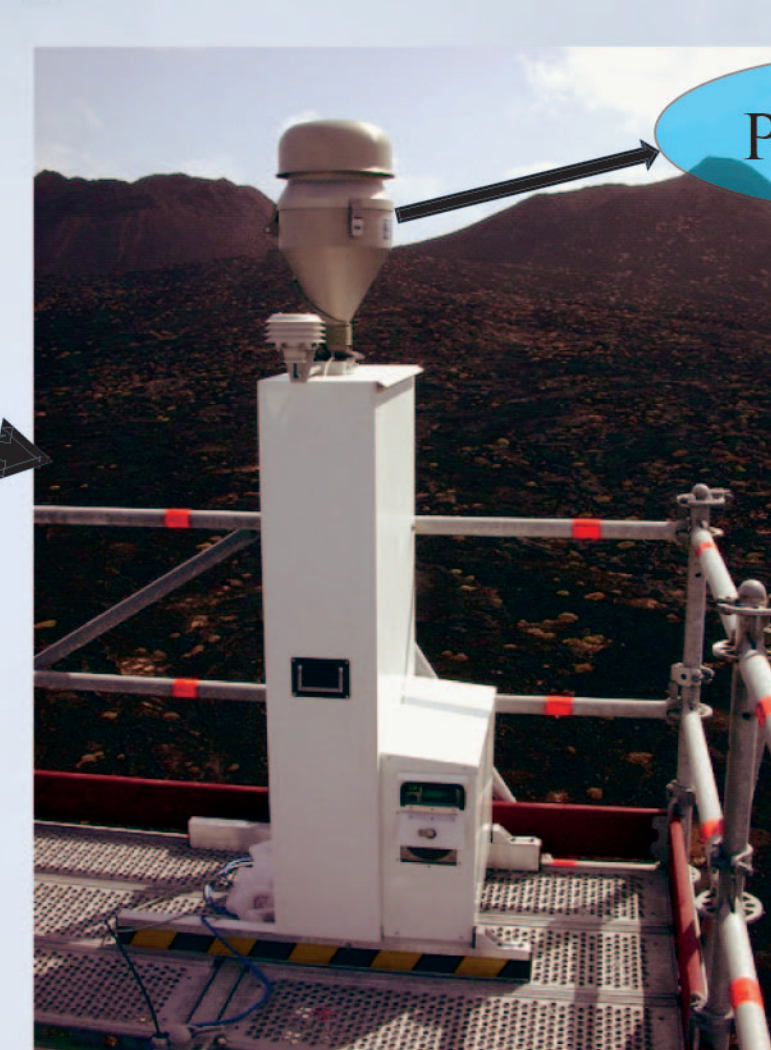
Fig.: DIGITEL DAH 80 high volume sampler equipped with PM 10 inlet.
