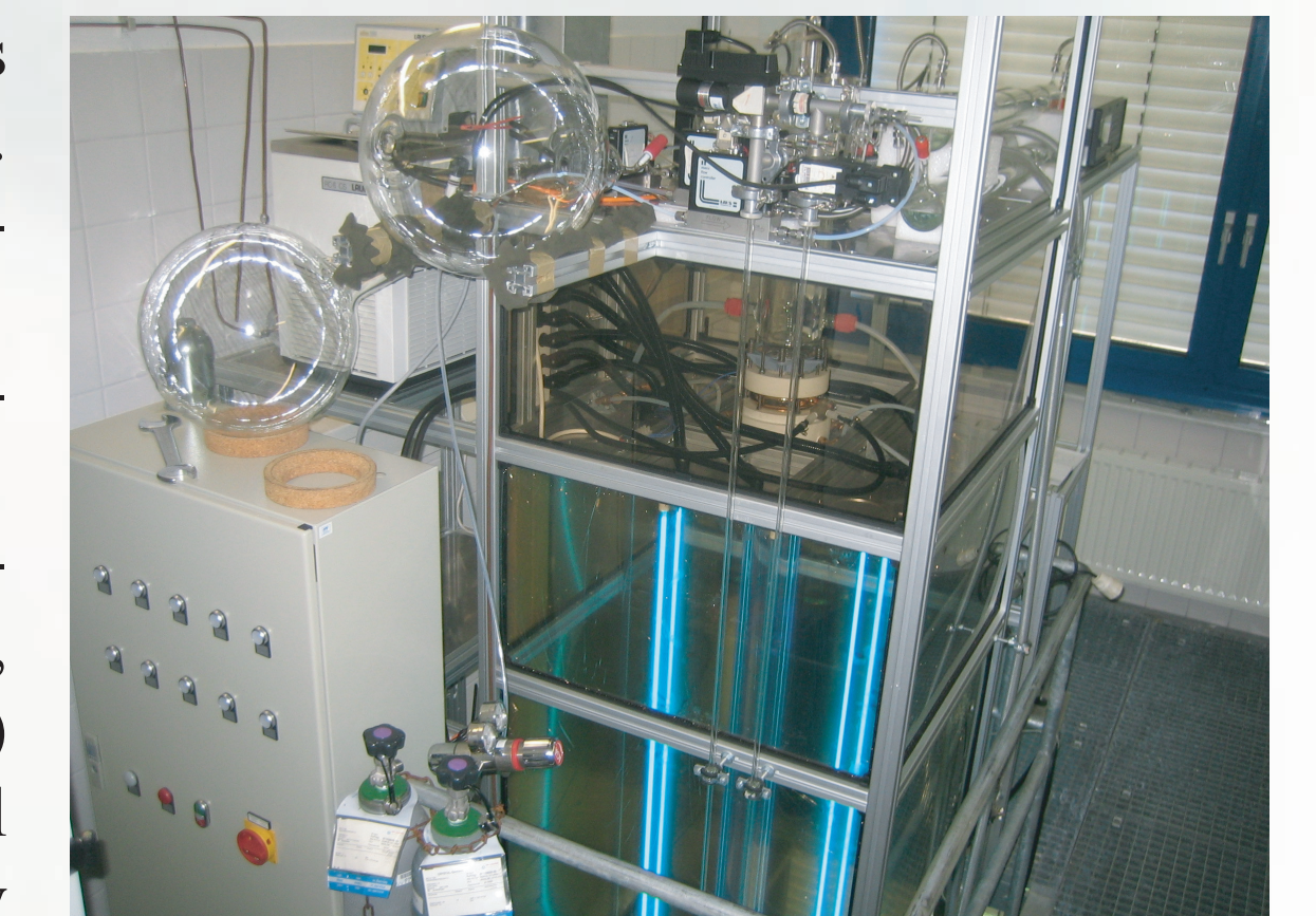
Head of the flow tube: Non-irradiated first section with the gas inlets as well as the gas mixing devices
