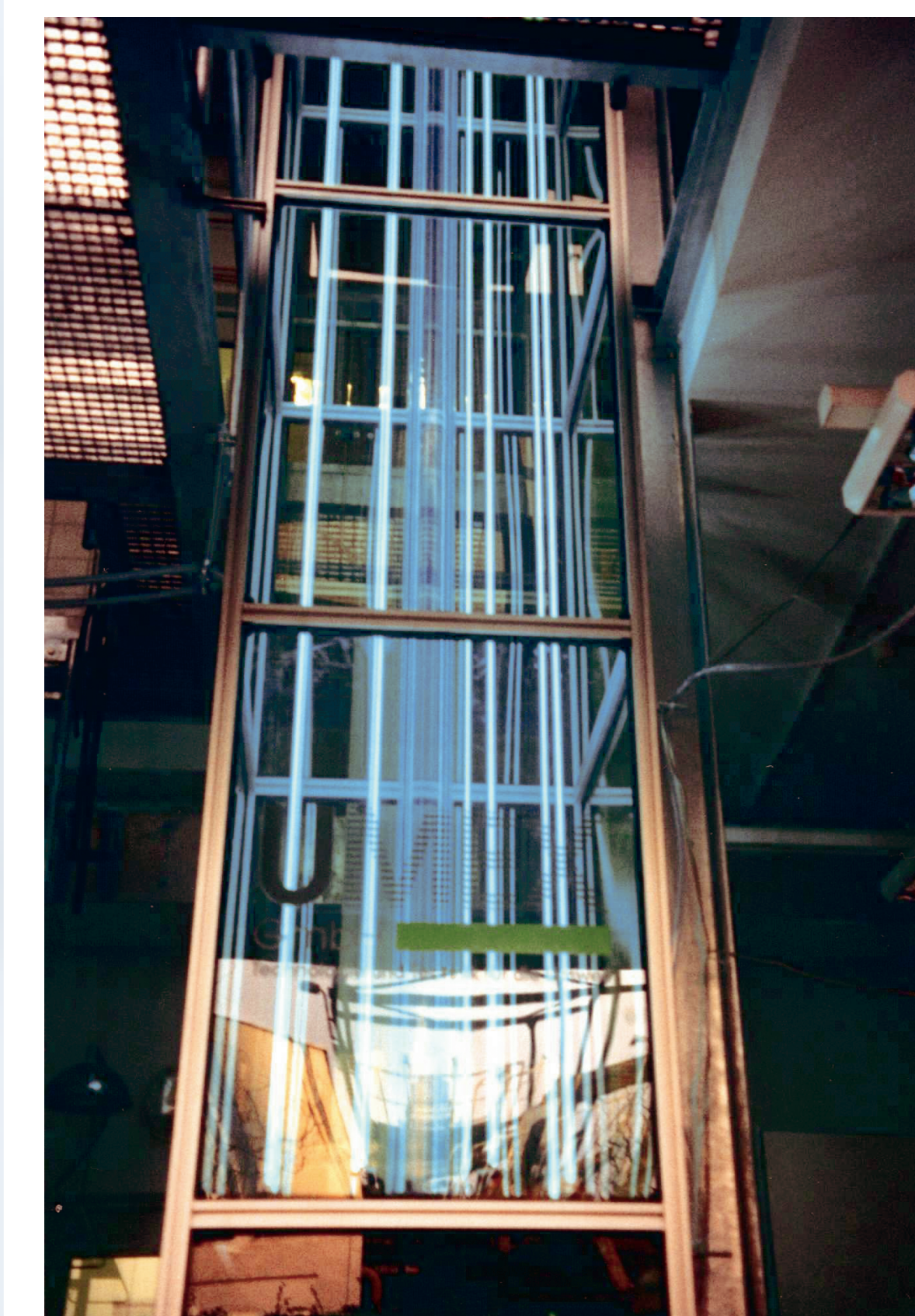
Fig. 1: The laminar flow tube, IfT-LFT
